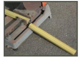
1. Amount to cut off shaft; Length of new shaft (step 2) Less groove to groove measurement (step 1); plus 76mm (3"). Cut this amount off both inner and outer drive tubes. Remove burrs and grease tubes.
