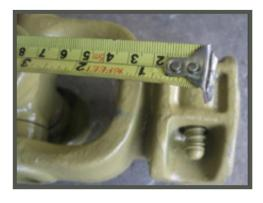
3. Required length of shaft is groove to groove length (step 1) less a minimum of 76mm (3") to allow for disconnection from tractor and prevent end thrust damage. If shaft is shorter than this, ensure that 50% of telescopic tubes over-
