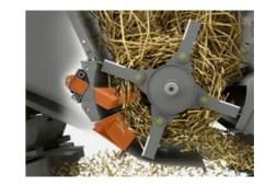
Static knife and pivoting bottom element in SPECIAL CUT chopper
