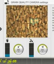
In order to help you adapt your machine to the ourrent harvesting conditions, CEMOS analyses the data from multiple sensors. The proportions of broken grain and non-grain determined by the GRAIN QUALITY CAMERA are important variables for optimisation. Please therefore ensure that the sensitivities for these two signals are set correctly by adjusting the sensitivities so that they match the displays showing the real conditions (camera image).
