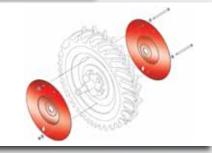
**Counterflanges** This optional feature protects the transmission wheels from impacts with stones.
