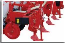
**Ridge planting** This system allows the ridge planting for irrigation.
