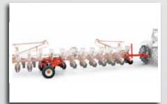
**Integrated cart** The transport cart allow an easy transport of larger rigid frame machines.
