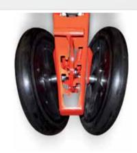
**Rubber Tire 2"** Standard 2" rubber-tire closing wheels suitable for conventionally tilled and loose soil. The soft rubber prevents soil from sticking in wet conditions.
