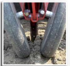
**Closing Wheels** Closing rear press wheels with sealed bearings and bolt through design.
