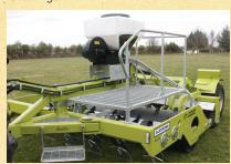
Large easy to access platform with safety rails for loading the seed hopper.
