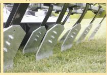
Wide profile flotation tyres on heavy duty hubs Individually sprung levelling boards for scratching the surface.
