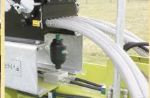
Hydraulic soft ride for dampening the hydraulics during road transport.
