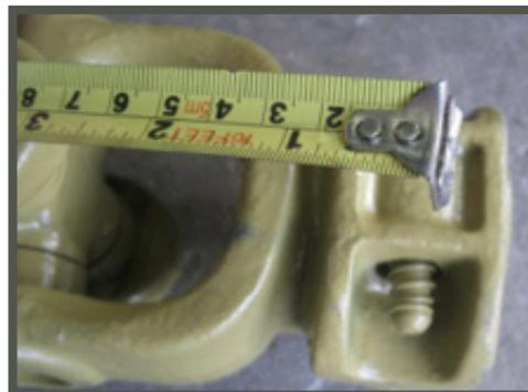
3. Required length of shaft is groove to groove length (step 1) less a minimum of 76mm (3") to allow for disconnection from tractor and prevent end thrust damage. If shaft is shorter than this, ensure that 50% of telescopic tubes overlap.
