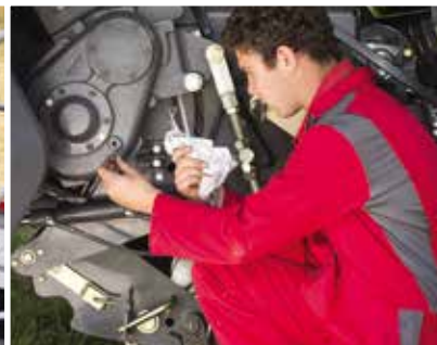
3. Checking the cutter gearbox oil level.
