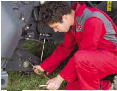
Three pre-set chop lengths can be easily selected using this selection rod.
