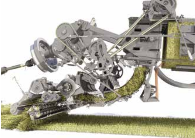
Pre-Compression Chamber – filling.
