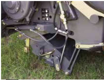
Lowering of the knife bed gives easy access to the knives and aids removal of foreign objects.
