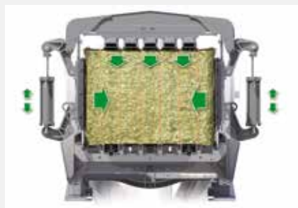
Three-way double acting density system.
