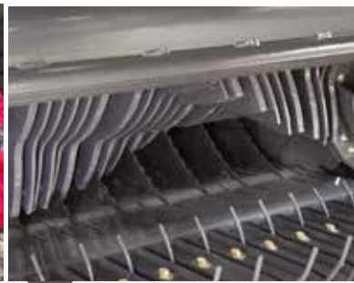
Heavy duty four-lobed spiral cutter rotor for smooth crop flow.
