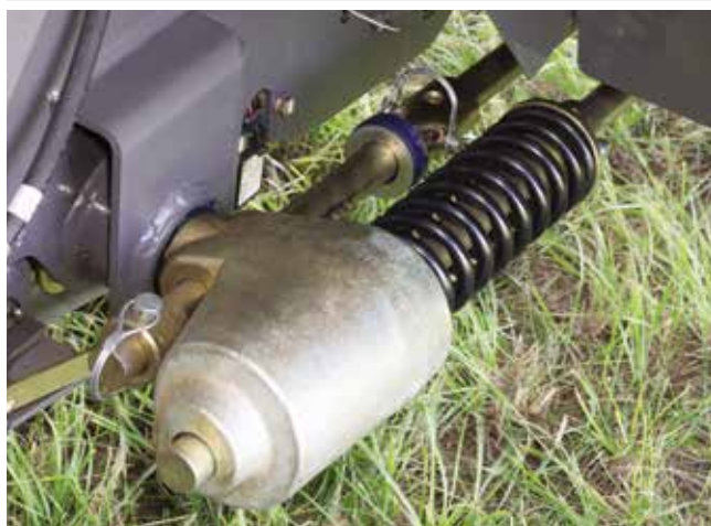
Compression spring pick-up suspension designed for high speed operation.
