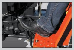
**Live PTO with Dual Stage Clutch** Depressing the clutch halfway will stop tractor's movement. Depressing the clutch all the way down will disengage the PTO. The new, larger diameter, dual stage clutch offers more durability and more power.
