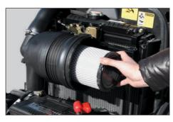
**Engine Air Filtration** The canister designed air filtration protects the engine from harmful dust and dirt, prolonging engine life.
