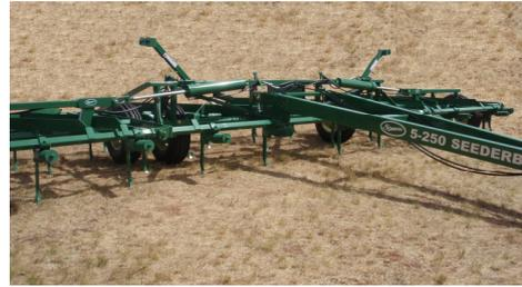
This machine has a five row 75mm x 75mm frame, dual walking wheels on the centre section and wings. (33t model, centre only), which are fitted with 10.00 tyres. (9.00 optional)
