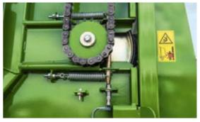
When the feed pressure is reached on the lower feed roller, the motion sensors stop the scraper floor feed automatically.
