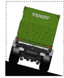
Without the automatic levelling control, the vehicle tilts downwards or to the side on slopes depending on the load and cornering speed (see Figure left). With the automatic levelling control from the FSC, the vehicle always stands parallel to the slope. The vehicle always adjusts to the best chassis height depending on the load (see Fig. right)
