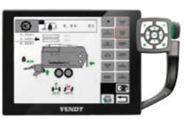
Control the bulkhead and the cutter unit on your terminal. Even the pick-up and drawbar can be conveniently adjusted from here.
