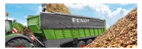
The Fendt Tigo is designed without a tubular frame to allow simple filling from above, whether using the bucket or the chopper.
