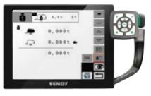
The weighing system optionally integrated at the hydropneumatic chassis suspension shows the crop yield to you comfortably in your cab. Thus, you maintain a constant control on the weight and the payload.
