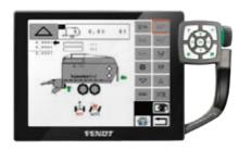
With TIM ready, the Tigo XR can adjust the speed of the tractor according to the swath strength and pick-up capacity.
