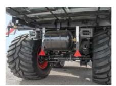
All models can be fitted optionally with hydraulic or electronic forced steering. The efficient, smart drawbar design also allows a steering angle of 60° even with forced steering.
