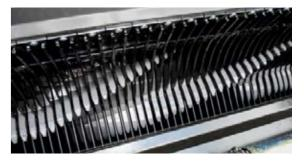
With a diameter of 800 mm and 7 spiral tine rows made of Hardox steel, the rotor is equipped on both sides with large spherical roller bearings.
