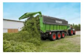
All wagons in the Tigo PR and XR series can be supplied either with 2 or 3 feed rollers. For more load volume, the individual rollers can be simply extended towards the back.
