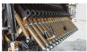
Use the FlexSharp knife sharpener to sharpen the knives without removing them.
