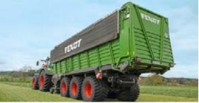
The hydraulic loading space cover is easy to operate via the terminal.
