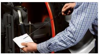
It's easy to check the transmission oil level at the rear.
