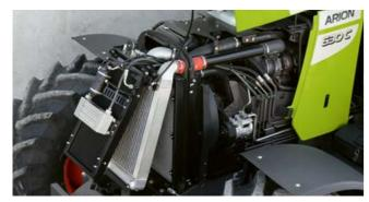
The radiator can be quickly tilted to one side for cleaning.
