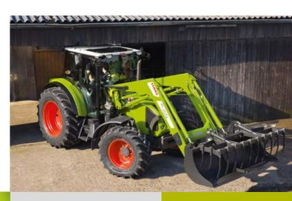
Pivoting front mudguards allow maximum steering angles.
