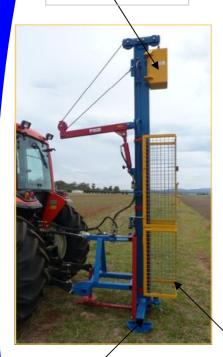
An adjustable sliding clamp is fitted to the main beam to keep post straight when driven
