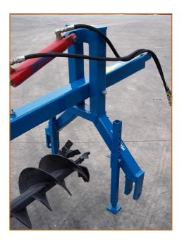
All Augers are fitted with the Pengo Boring Head with replaceable earth teeth at 35° angles and bolt on pilots. All augers have a double cutting head. Optional teeth and pilots are available to suit various ground conditions.
