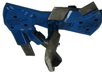
**Old cutting edges (fan or segment shaped)**
