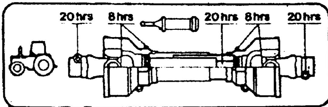
FIGURE 2. : Grease points and intervals for P.T.O. shaf
